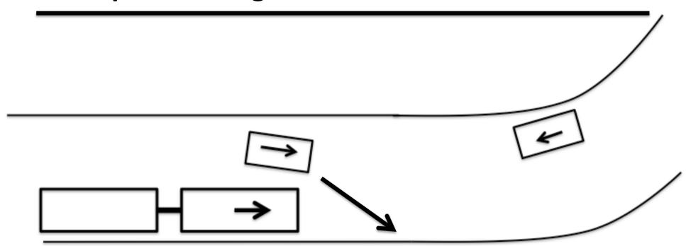
**Strategy (a)**: accelerate further to finish the passing maneuver quickly and aligns the car ahead of the truck. **Strategy (b)**: perform an emergency braking action and align the car behind the truck.
